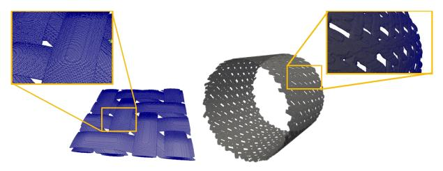
Figure 1: One layer triaxial 12k braid RVE model (left), 3D near-net-shape triaxial 12k braid model (right)
