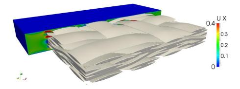
**Figure 2:** Viscosity field  $U_x$  of three layered triaxial 12k braid (RVE)
